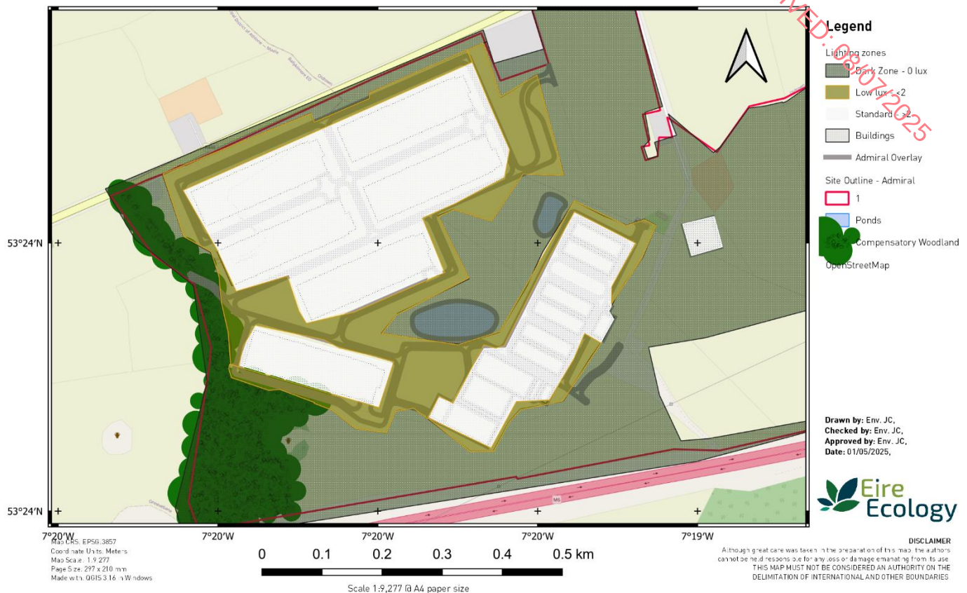
Figure 6-3: Section 1 lighting zones
